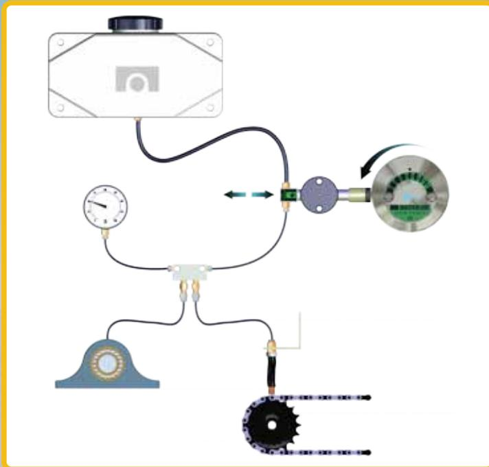
Meter units ensure each point receives the correct ratio of oil
