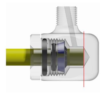
2. Ensure Pipe fully located into fitting.
