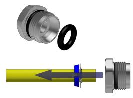
3. Remove o-ring from Sleeve nut, Introduce chamfered end of the sleeve nut the to star washer at other end of pipe.
