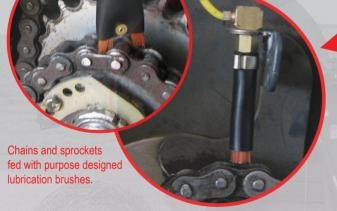
Constant oil lubrication is safer, reduces machine downtime & can considerably extend component life
